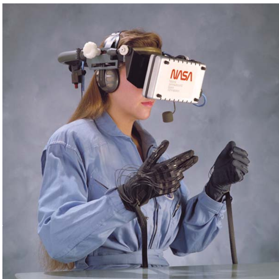
Figure 3. The Virtual Interface Environment Workstation (VIEW), 1990. Photo credit: NASA/S.S. Fisher, 1989.
