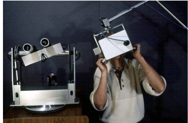
Figure A10. VIEWlab remote controlled stereoscopic telepresence camera system. Photo credit: NASA/S.S. Fisher, 1988.
