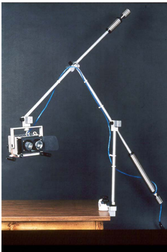
Figure A9. VIEWlab counterbalanced CRT-based stereoscopic viewer (CCSV). Photo credit: NASA/S.S. Fisher, 1988.
