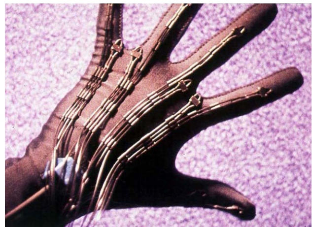
Figure A11. VIEWlab fiberoptic dataglove prototype, 1987. Photo credit: NASA Ames Research Center, 1987.
